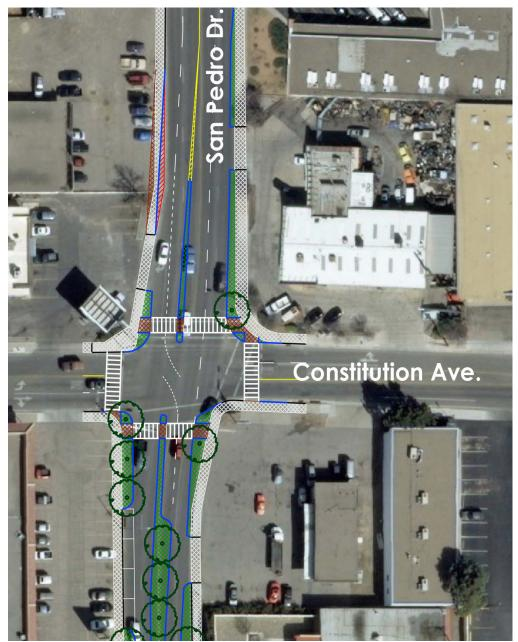
Figure 3.3: "Straightened" Constitution intersection. This proposed alignment would reduce the angle of the intersection from 8 degrees over 200 feet, to 4 degrees over 400 feet.
